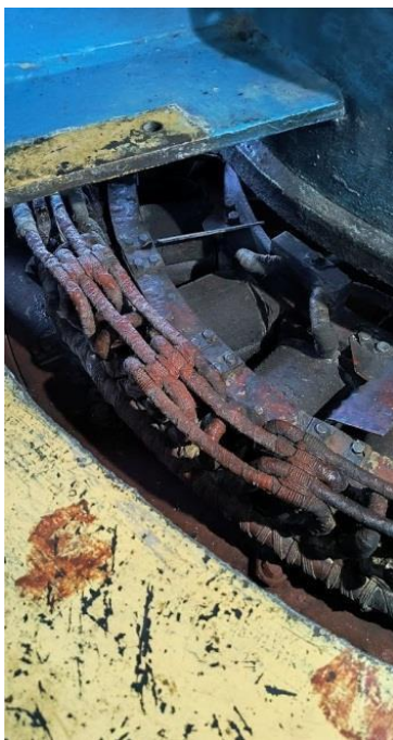
Figure 3-3 Examples of corroded windings in worn out electric motor
